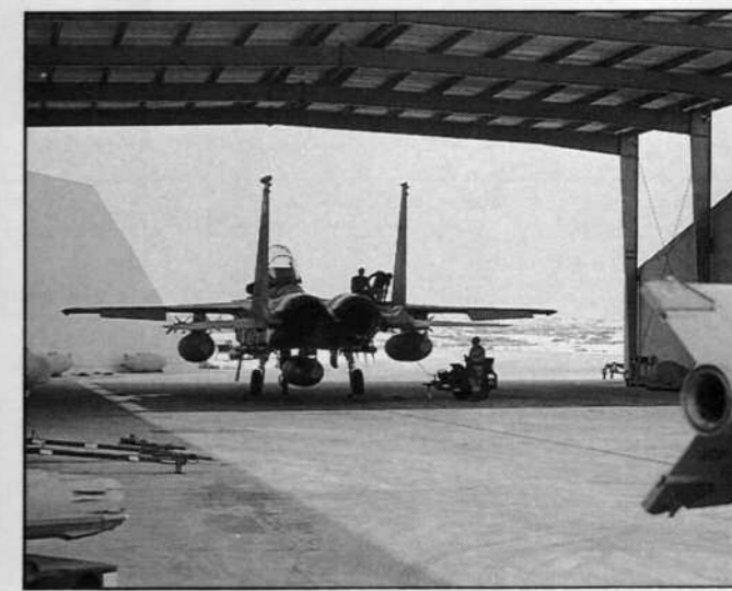
■ A fully loaded F-15, carrying eight AAMs and three external tanks, stands under an aircraft shelter in the munitions preparation area. (Photos: Ian Bennett).
